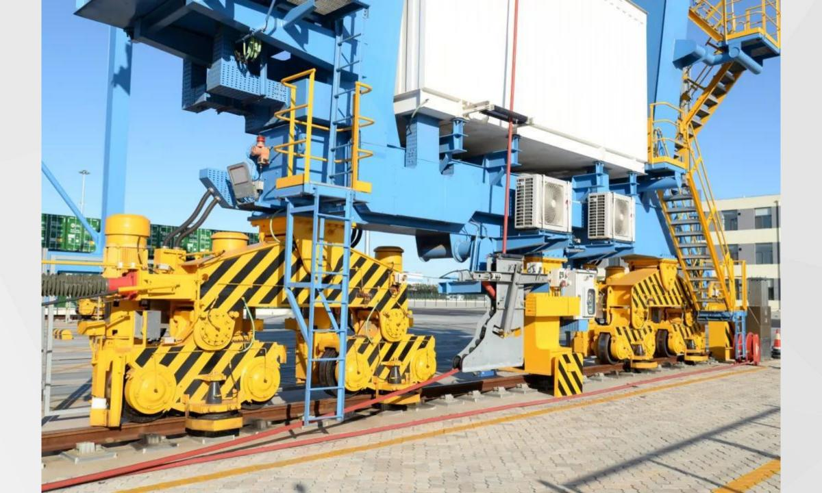
(5) The non-equal-length rear-extension double-trolley bridge crane is first created, which reduces the requirement of foundation bearing capacity and optimizes the layout of bridge crane.
